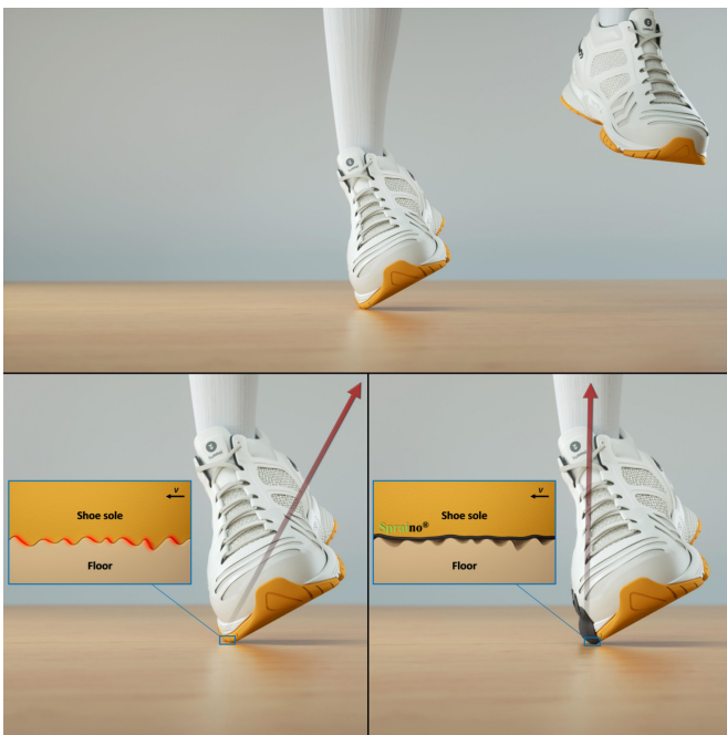
Figure 2 Preventive mechanism of Spraino: in case of a bad landing, Spraino minimises the otherwise high shoe–surface friction at the lateral edge of the shoe. This minimises the horizontal ground reaction forces (GRFs), thereby bringing the GRF vector closer towards the joint centre which serves to prevent excessive ankle inversion and internal rotation.
